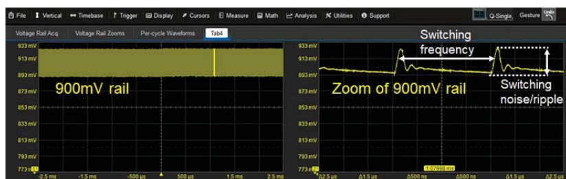
1. Zoom lets you examine noise and ripple on a 900-mV power rail.
