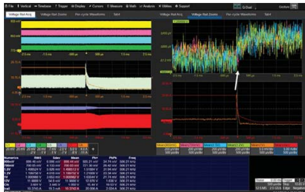
7. A load release on one power rail has minimal effect on other power rails.
